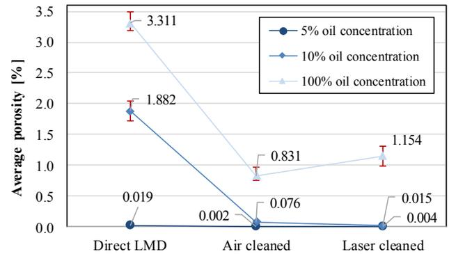
Fig. 8. Average porosity attained for each test.
