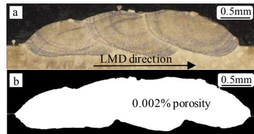
Fig. 1. Reference test (a) metallography; (b) average porosity results.
