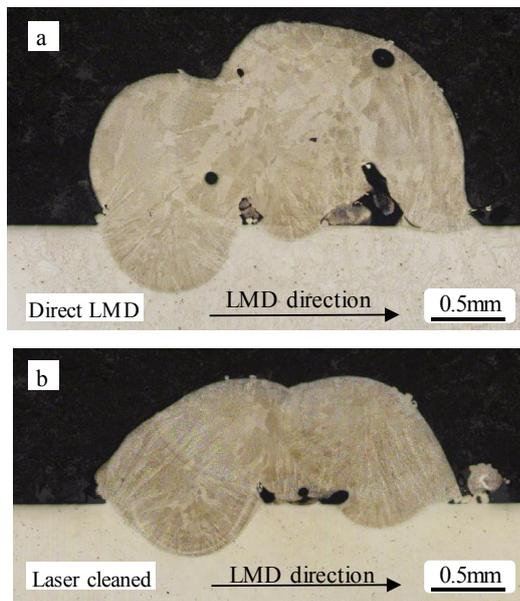
Fig. 7. 100% concentration tests (a) direct LMD; (b) laser cleaned.
