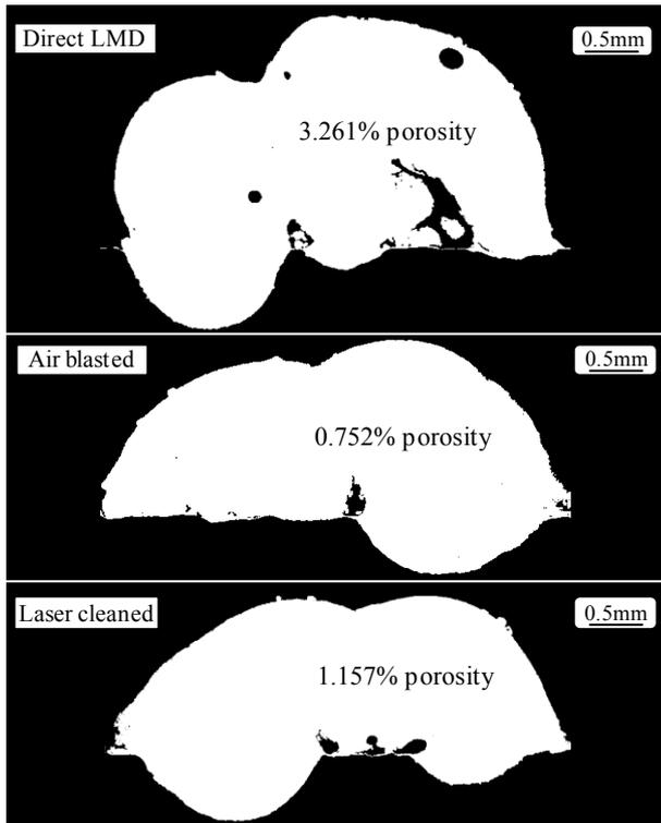
Fig. 6. 100% concentration tests porosity results.
