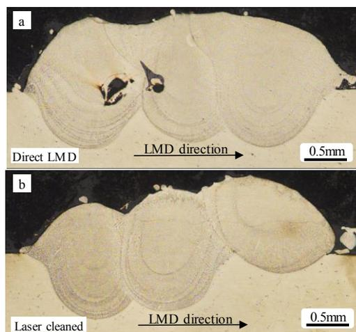
Fig. 5. 10% concentration tests (a) direct LMD; (b) laser cleaned.
