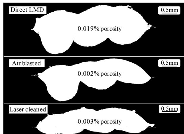
Fig. 2. 5% concentration tests porosity results.
