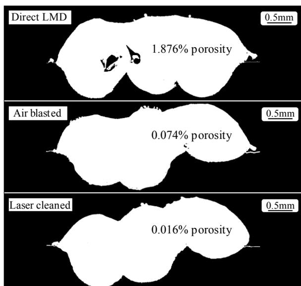
Fig. 4. 10% concentration tests porosity results.
