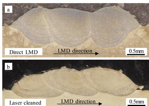
Fig. 3. 5% concentration tests (a) direct LMD; (b) laser cleaned.
